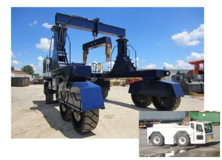
The Vertical Cask Transporter (top photo) that will be used for outdoor transport of HLW storage casks at the West Valley Demonstration Project and the tow tractor that will pull it are pictured above.
