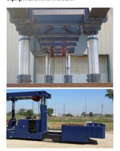
Robust hydraulic cylinders (middle photo) and extendable rear counterweights (above) will accommodate heavy lifting.
