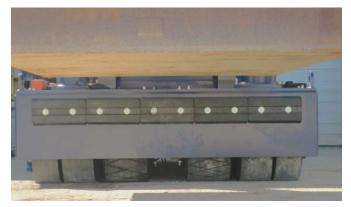
The TL220's wheel configuration is designed to distribute the weight of HLW storage casks.
