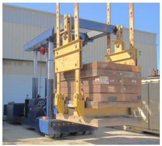
A load test of the TL220 in progress.
