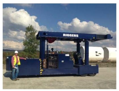
The TL220, pictured above, is one of three transporters that were specially-designed for lifting and moving HLW storage casks.
