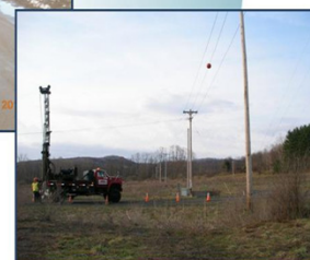
Geotechnical studies have been conducted along the site roadway
