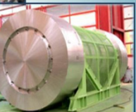
The fully-loaded pad will appear similar to the SNF storage pad shown above. The HLW Overpacks are designed for off-site transport via NAC's Storage and Transport Cask, pictured at right.
