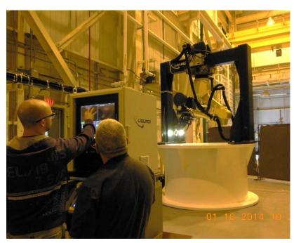
The HLW Overpack Automated Welding System is pictured above in a mockup used for operator training.
