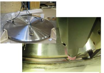
The Overpack lid (top photo) will be welded in place to provide a secure shipment-ready package.
