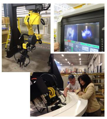
The Automated Welding System (top left); The weld is viewed and recorded on a display terminal (top right); and a close-up of the arm and welder head in a welding mockup (above).
